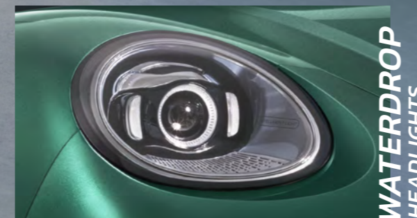
Signature LED water droplet design, with smart auto on-off.
